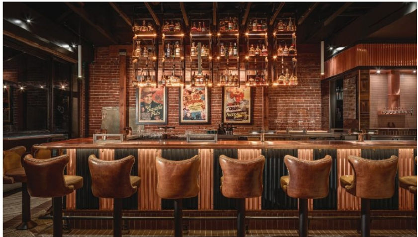
Cantilevered robotic shelves above the bar raise and lower as needed for service and stocking. Finished to blend in with the ceiling when raised, the six three-shelf units are lit to illuminate the bottles and can be activated individually or as a group by bartenders via motion sensors.
