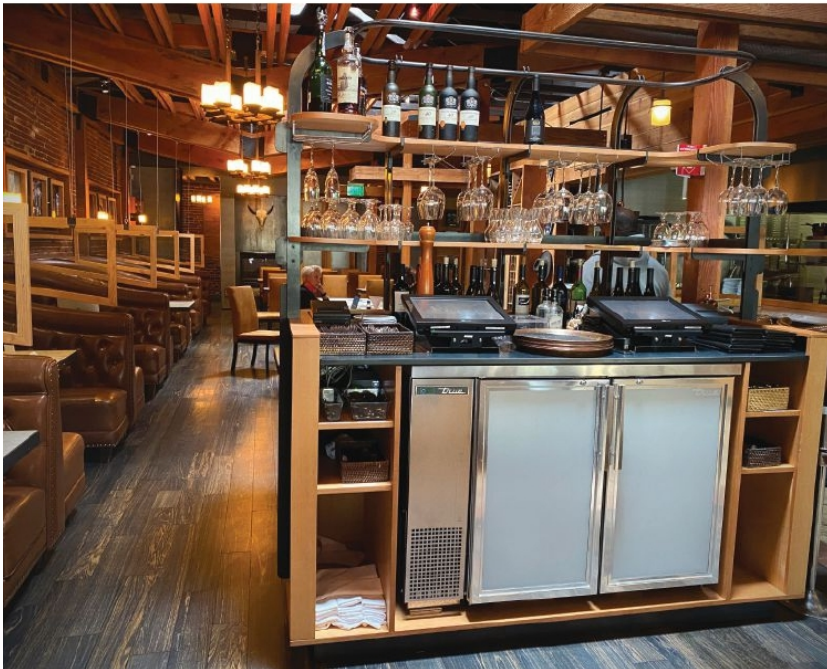
A wall with banquette seating that used to separate the bar from the dining room was replaced with a new, open-shelf server station that provides for better sight lines into the restaurant.
